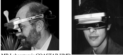
MR Laboratory's COASTAR HMD (Co-Optical Axis See-Through Augmented Reality) Parallax-free video see-through HMD
