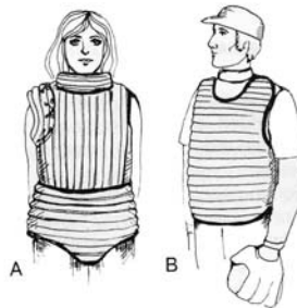
Segmented body padding. A, a woman's softball protector segmented vertically on top to conform to the female anatomy and horizontally below to accommodate the crouched position of the catcher behind the plate; B, a typical catcher's chest protector for men.
